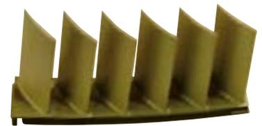
Applied and processed typically as per RPS 666/5. Note that Smoothseal is normally cured at 250°C to retain the golden finish. Normal film thickness 3-5 microns applied in 3-4 very thin coats.
