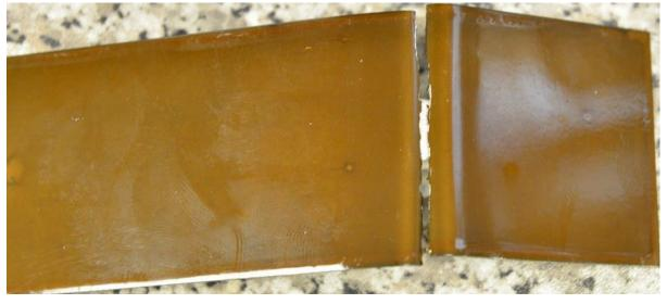
**Salt Spray:** ASTM B117 – neutral hot salt spray. 200 hours unbroken exposure. Substrate – Magnesium
