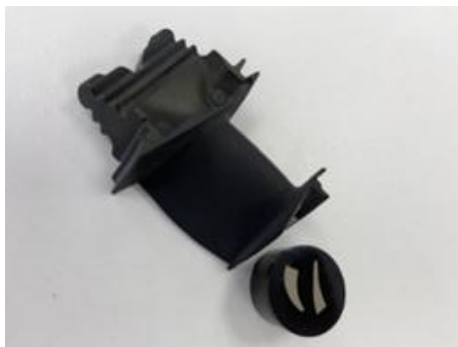
CFIPAL coated part with example of a typical cut through
