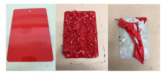
The above pictures show the effect of IPSTRIP-500, when applied to an aluminium panel, coated with IP9064-5380 to a thickness of 50 microns, which was fully oven cured prior to stripping.
