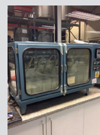
▶ Sietam Cabinet for testing to EN 3212.
