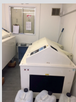
▲ 100% Humidity Cabinet for testing to ASTM D2247 or BS3900 F9.
