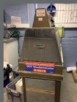
BSENISO 11507 QUV BS3900-F16 accelerated weathering cabinets
