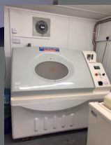
Salt Spray Cabinets for testing to ASTM B117.
