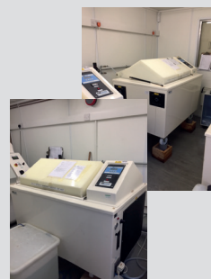
▶ Sand Erosion Cabinet for testing to MSRR9910 Test 22 with separate ASTM D968 Sand Abrasion tester.
