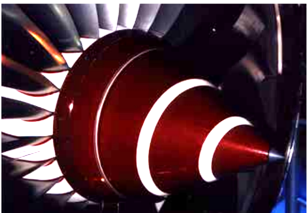
Engine nose cone coated with 2 component sealer plus EROS Elastomeric top coat.
